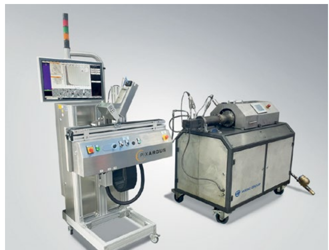
The Technical Center of the HF Mixing Group features two larger lab-scale mixing lines. For quality control, the compound mixing experts use inspection technology from PIXARGUS (Photos: HF Mixing Group)
