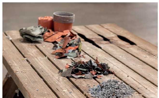
Flower pot recycling cycle: raw material, flakes, & granules
