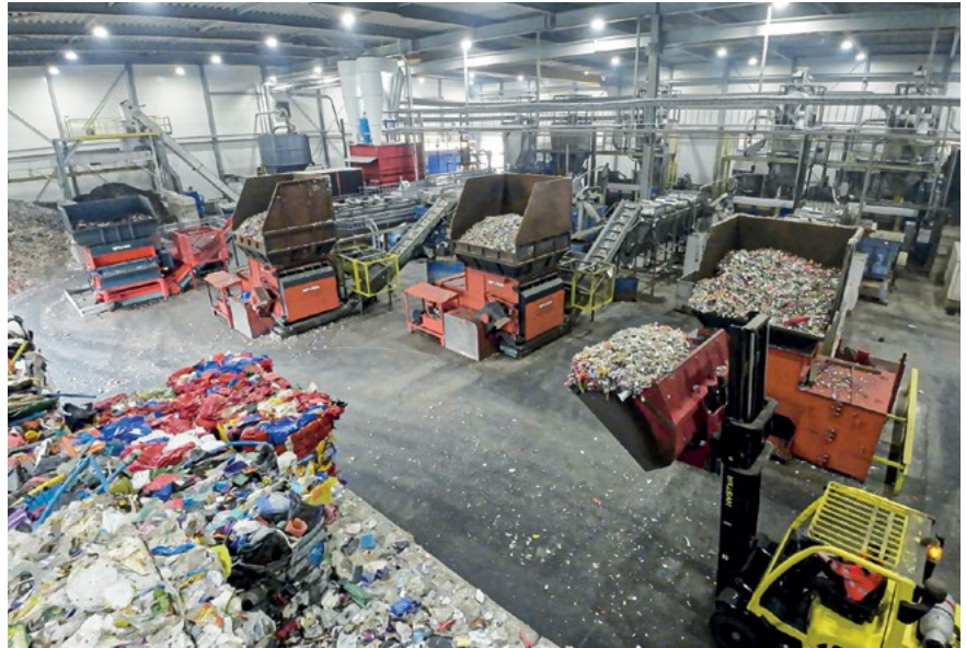
Shredder quartet: The WEIMA W5.18 single-shaft shredder
