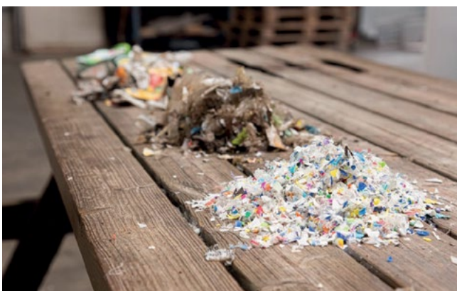
Recycling cycle of post-consumer plastics: raw material, flakes, & granules
