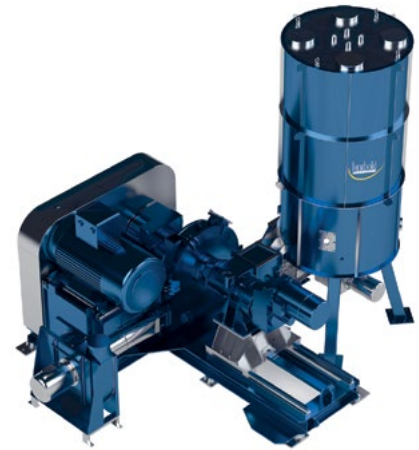
The HV 70 plastcompactor is the most powerful of the series from Herbold Meckesheim. It processes the feedstock in continuous operation between a rotating and a fixed compactor disk, which are equipped with screwed-on and easily exchangeable kneading bars (Photo: Herbold Meckesheim, Meckesheim, Germany)
